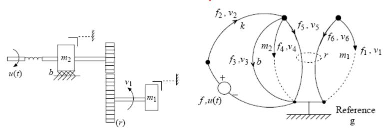
**Rotary-Motion System with Velocity Source and Gear Transmission; Linear Graph**
