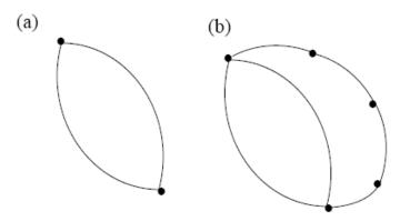
**Step 1:** Start with Graph (a):  $\ell = 1, b = 2, n = 2 \leftarrow (i)$  is satisfied. Add new loop by using *m* nodes and m + 1 branches, as in Graph (b)  $\ell \rightarrow 2; n \rightarrow 2+m; b \rightarrow 2+m+1 \rightarrow (i)$  is still satisfied *Note:* m = 0 is a special case
