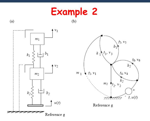
Main System  $(m_2, k_2, b_2)$ ; Dynamic Absorber  $(m_l, k_l, b_l)$ ; Velocity Source u(t)# branches = b = 7; # nodes = n = 4; # sources = s = 1# independent loops = l = 4; # unknowns = 2b - s = 13# constitutive eqns = b - s = 6; # node eqns = n - 1 = 3; # loop eqns = 4 Check: # Unknowns = 2b - s = 13; # Eqns = (b - s) + (n - 1) + l = 6 + 3 + 4 = 13
